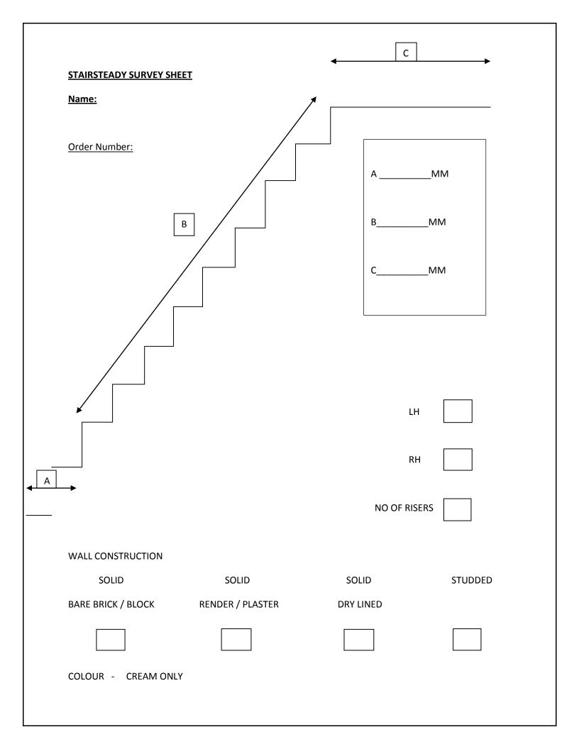
MEASURE THE DISTANCE FROM THE GROUND FLOOR WALL TO THE FIRST RISER, PLACE THIS MEASUREMENT IN MM ON THE SURVEY SHEET AS **A**.
